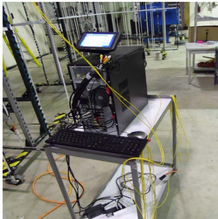
Figure 5.8 The multi-functional portable FLRD control device.
