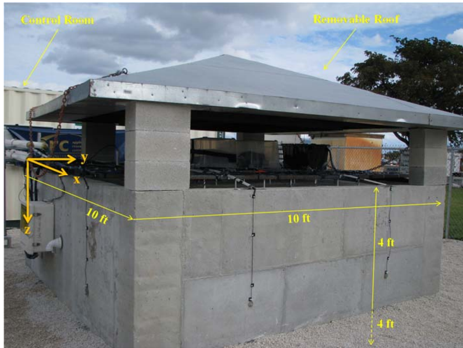
Figure 5.7 The concrete test cube filled with grout, and ready for testing.
